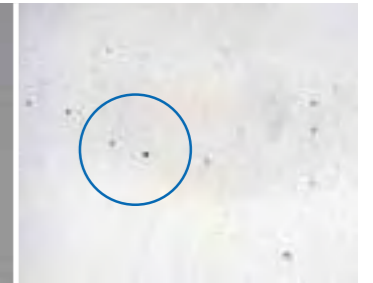
Thermal wall bullet exit side, exit hole as big as a pin head
