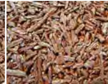
Bullet exit side in 7 cm thick Regupol, no wear visible!
